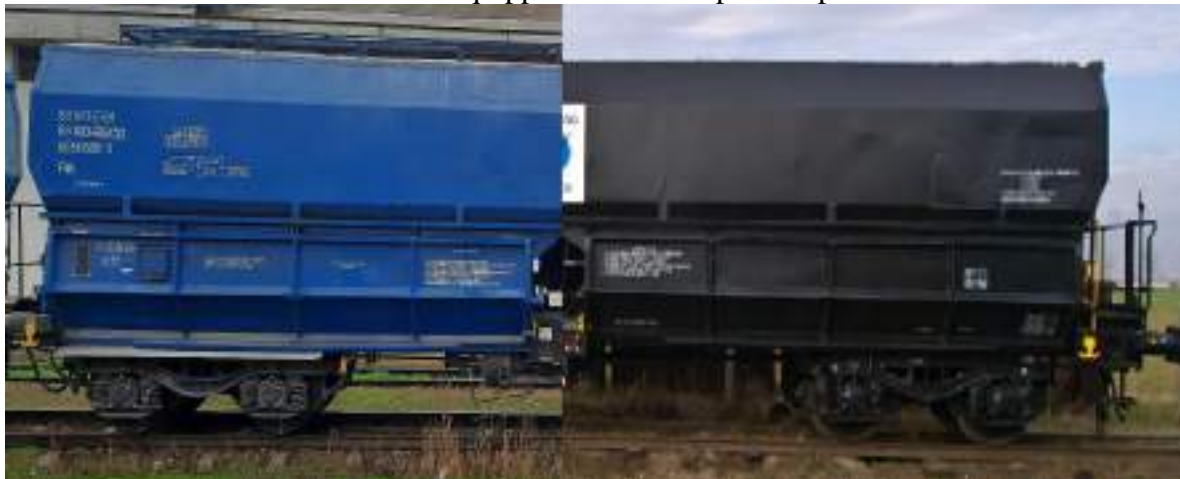
Photo no. 9 – Fals series wagon with fixed downgrade (bottom) compared with standard Fals series wagon (top).
