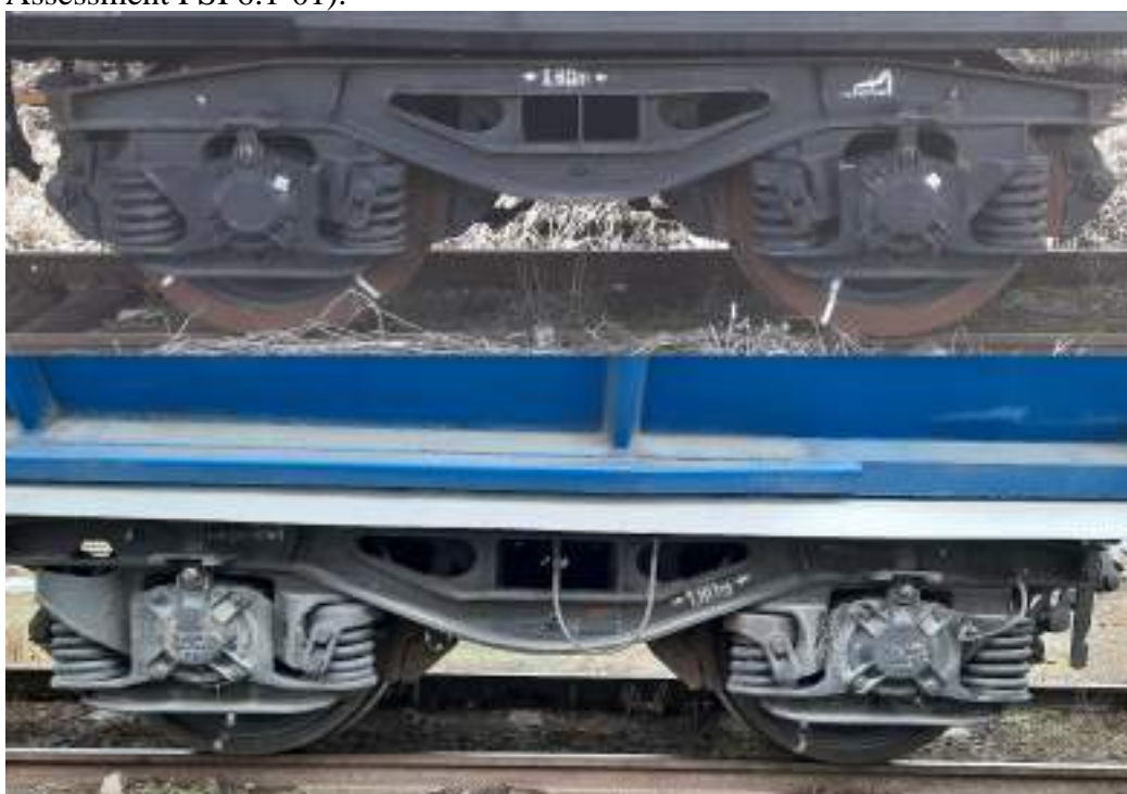
Photo no. 10 – Comparative view of access to the side bearers: standard Fals series wagon (top) vs. Fals wagon with fixed downgrade (bottom).
