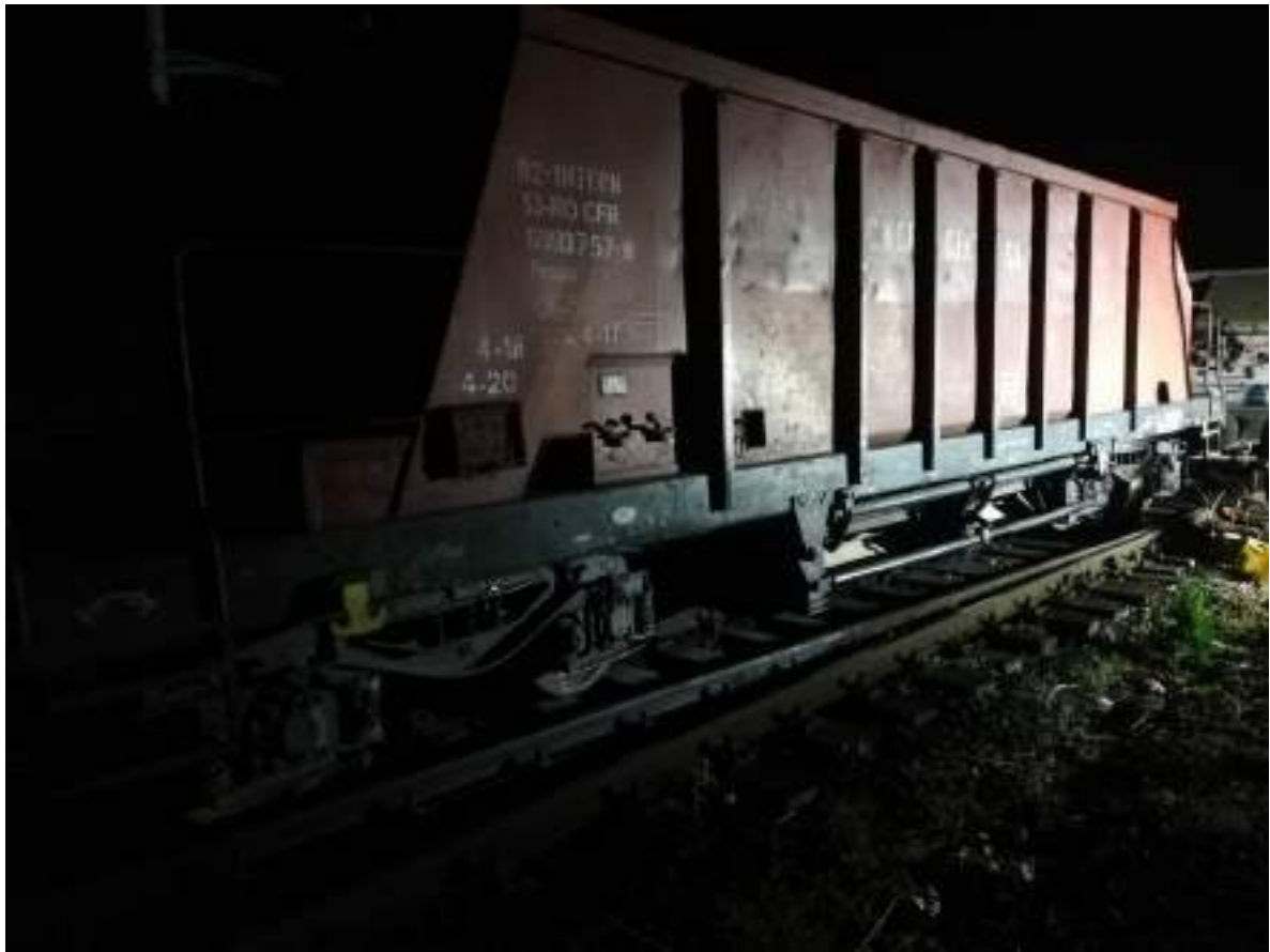
Photo no.1: derailed wagon no.82536993757-8 (photo taken from the right lateral side in the running direction)
