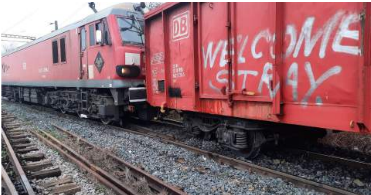
Photo no.1: the wagon no.33535421218-5, derailed
