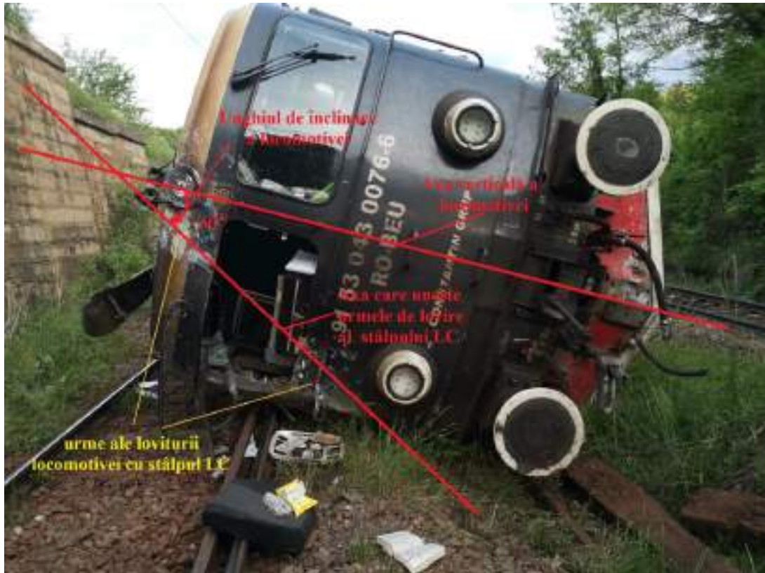
Figure no.6 – establishment of the locomotive reclining when it hit the first pole of the contact line
