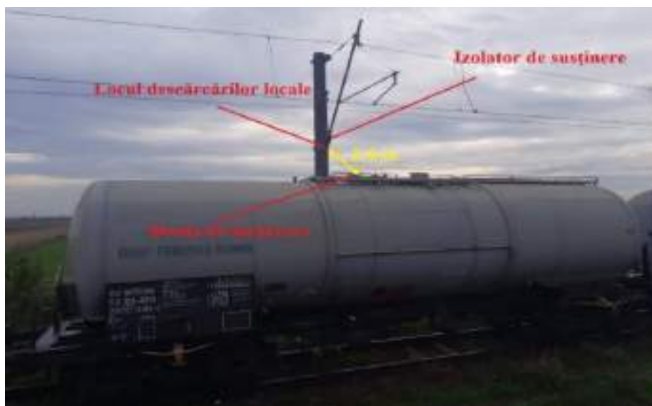
Photo no. 14 – site of local discharges, support insulator, distance from the loading dome of the wagon to the insulators for the support of the contact line, loading dome
