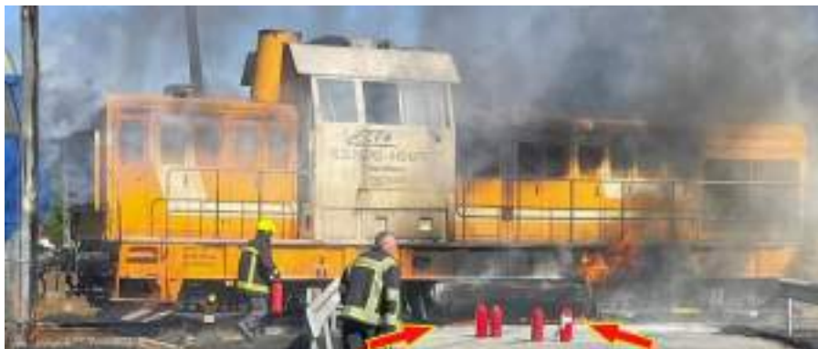
Photo no.31 – during that time the diesel fuel burnt under the tank (photo taken by a witness)
